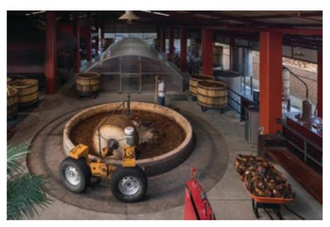
Rather than using a donkey to pull its heavy mill wheel, Sombra's distillery is outfitted with rooftop solar panels that power a mechanical tahona.
